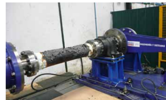
Composite shaft testing after fire
