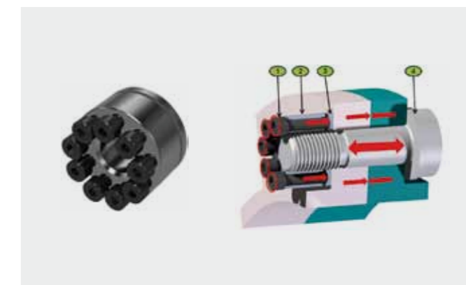
Super Nut principle
