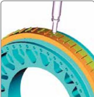
Powerlign/Powerwheel pick up teeth shown with one sensor (second not shown is at 180°.)
